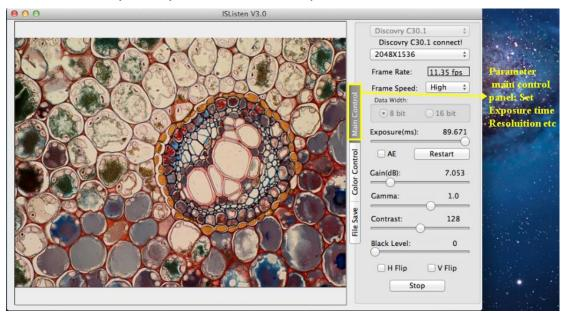
5. Click on "Color Control" tab to open the color parameter setting panel. In this panel, you can do the white balance or manually adjust the image color.
