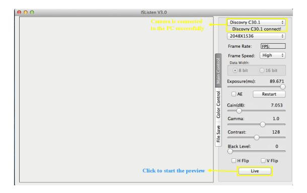
4. When start the program, it shows the software "Main Control" panel. You can set the resolution, frame speed, exposure time etc on this panel.
